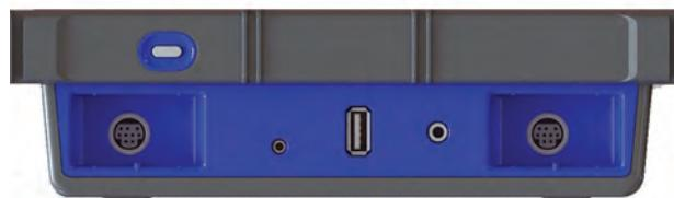
The SPARK LXi2 features two PASPORT ports as well as ports for the included temperature and voltage probes.
