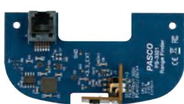
The Range Finder Module gives the PASCObot sight, allowing it to locate, avoid, and respond to objects based on code.
