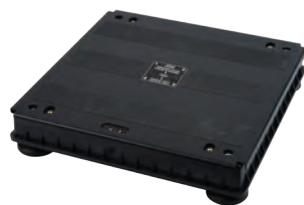
*The 2-Axis platform measures both the normal and parallel forces acting on the platform simultaneously. Determine the static weight of a structure or person, measure forces associated with the impacts of falling objects, and determine the dynamic vertical and parallel forces that arise when moving or jumping.*
