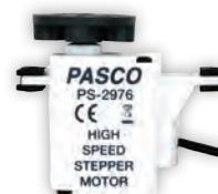
The PASCObot's motion is controlled by two Stepper Motors, which connect to the bot's Wheels. Compatible with other STEM Sense products, the Stepper Motors can be controlled individually to move the bot forwards, backwards, and around corners and curves.
